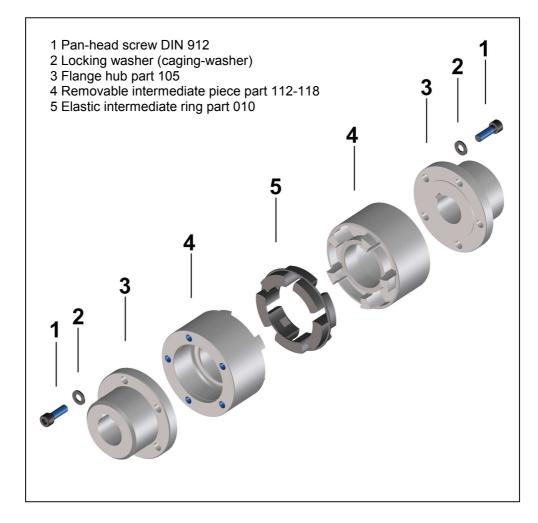
Fig. 1 Construction RINGFEDER® TNM H
